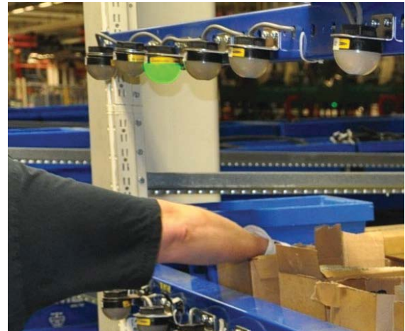
Figure 5. Pick-By-Light, an example of cognitive automation, LoA_{cog}=5
