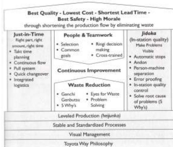
**Figure 1. The Toyota Production System as a temple with continuous improvement as driver [4]**
